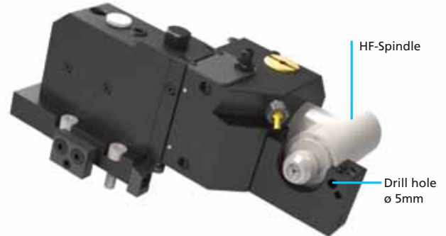
GWS-tool holder for counter spindle machining for angular HF-spindle ( \varnothing 25 or 30mm) and interface for 1 tool with shank \varnothing 5mm
