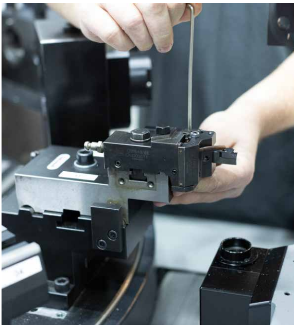
Convenient tool presetting outside the machine
